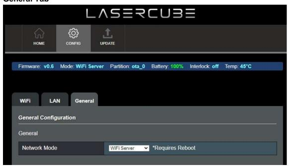
The network operating mode can be set from the drop down tab. The LaserCube will reboot after changing the mode.
