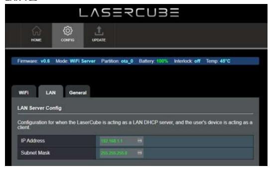
The IP address and subnet can be set for when the LaserCube is operating in LAN Server mode, where it provides a DHCP service.
