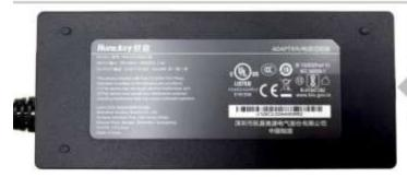
MODEL: HKA12019063-68 INPUT: 100-240V ~ 60/50Hz, 2.0A OUTPUT: 19.0V === 6.32A, 120.08W This device complies with Part 15 of the FCC Rules. Operation is subject to the following two conditions: (1) This device may not cause harmful interference,
